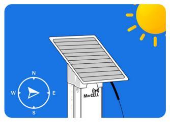
Direct the solar panel towards the East. The objective is to ensure that the solar panel receives direct sunlight early in the morning, allowing it to recharge the battery after the overnight usage.
