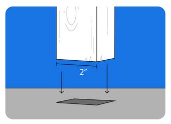
Insert the stake into solid ground, leaving approximately 3 feet above ground.
